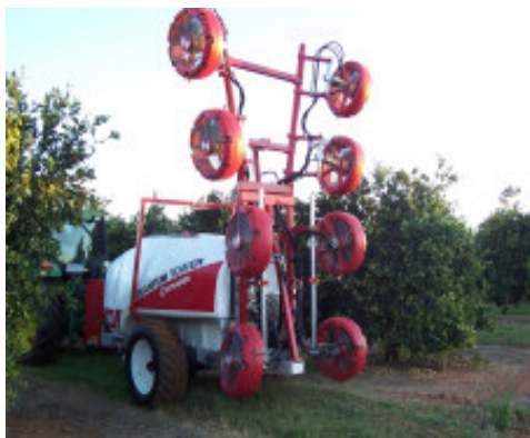
The new Croplands Quantum Mist sprayer for citrus uses SARDI fan technology
